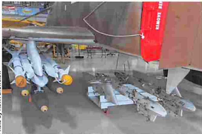
Multiple Ejector Racks (MERs) and pylons under the Phantom
